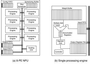
Figure 5: Reconfigurable 8-PE NPU.
