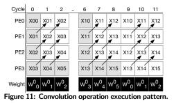
**Reusing data across convolution kernels.** Using the sequence of operations in Figure 11, the four PEs compute four adjacent output elements using the first kernel ( $Weight^0$ ).
