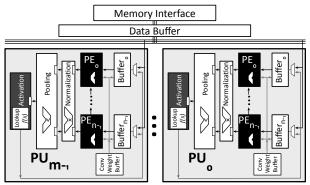
Figure 5: Overview of a clustered hierarchical template design. The template accelerator is divided into Processing Units (PUs) that are comprised of multiple smaller Processing Engines (PEs).
