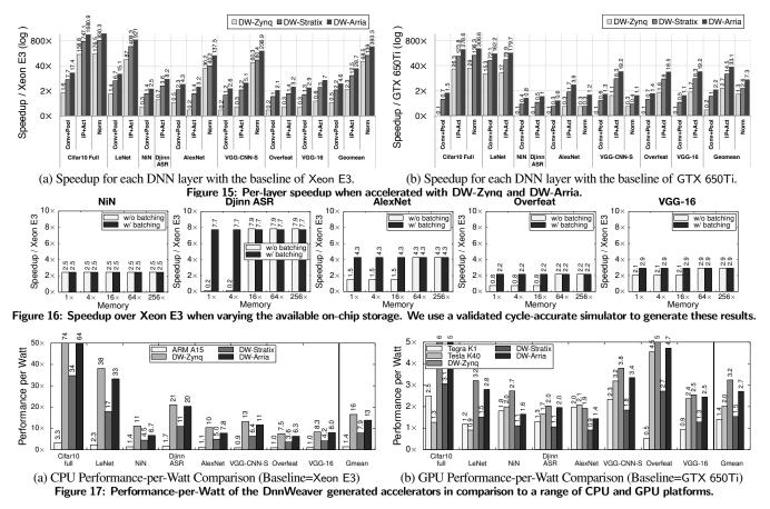
$13.9 \times$  higher performance-per-Watt than the baseline. Note that although DW-Stratix provides about  $10 \times$  higher speedup, the increased power consumption by DW-Stratix (2W vs. 25W) leads to the lower performance-per-Watt than DW-Zynq. However, DW-Arria provides higher performance that DW-Stratix, without a commensurate increase in power consumption, leading to higher performance-per-Watt. This trend is observed for all the evaluated DNN models.
